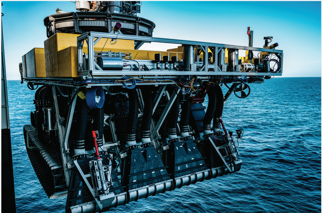
The Allseas-designed, pilot-scale nodule collector vehicle undergoes drive testing in the North Sea.
